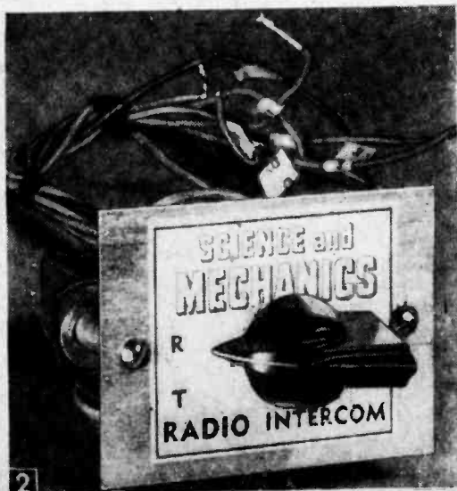
Close-up of intercom unit. Switch in R position for listening; turned to T for talking.
