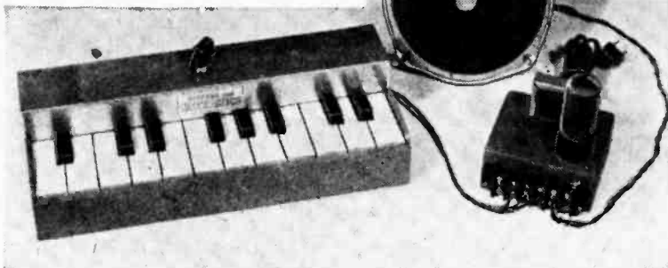
Completed electronic organ consists of: left, 20-key console with control providing 4 tone ranges; center, 5 in. PM speaker; and right, 1-tube oscillator.
