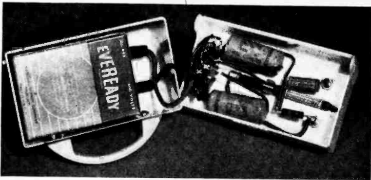
Detector case is opened to show location of components. Two capacitors (right) enable 300 volt battery to deliver 900 volts.
