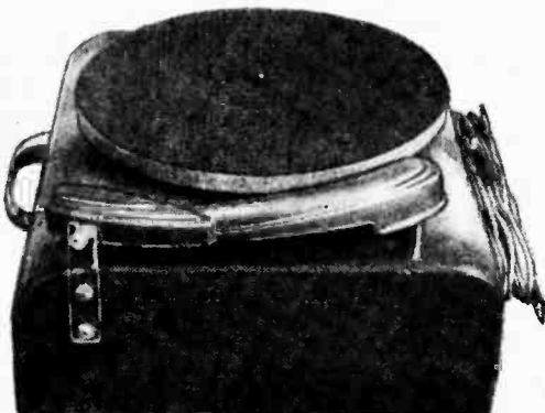
Fig. 2. AFTER—all dolled up! Note chrome handle, layer of felt on hard turntable, arm rest and lock, and brackets for reeling up line cord and pickup cable.
